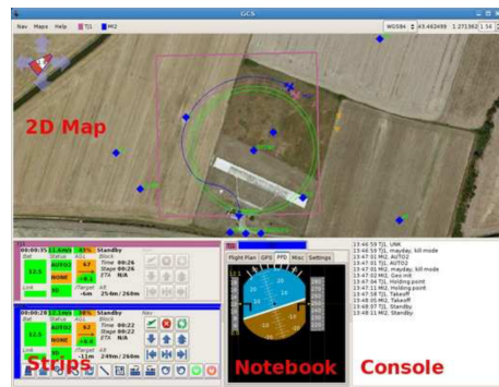
Figure 3: Ground Control Station Graphical User Interface [10].
