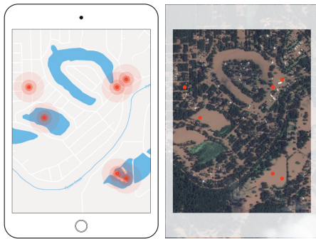
Figure 5: During catastrophes map material can differ drastically from the situation on site. Therefore, the assignment of drones indicated on GUIs with drones seen in the field may turn out to be difficult to almost impossible. Selecting drones with gaze could turn out to be beneficial in such situations.
