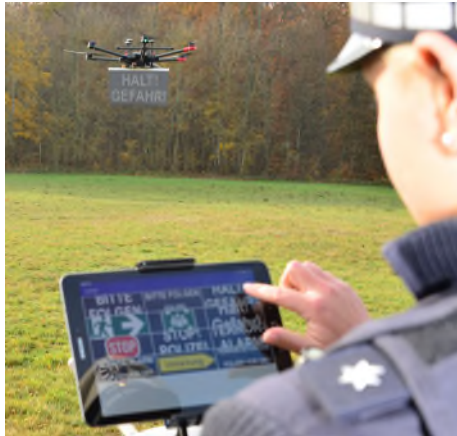
Figure 6: A police officer uses the tablet computer to dynamically control the content of DisplayDrone.
